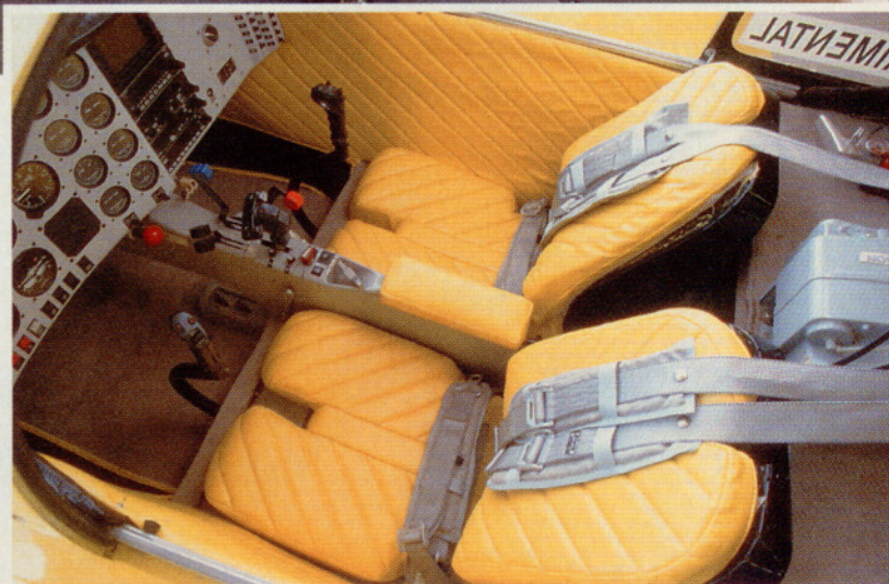
The number of switches on the throttle and stick has been reduced to prevent confusion. The throttle is like that of a modern fighter.
